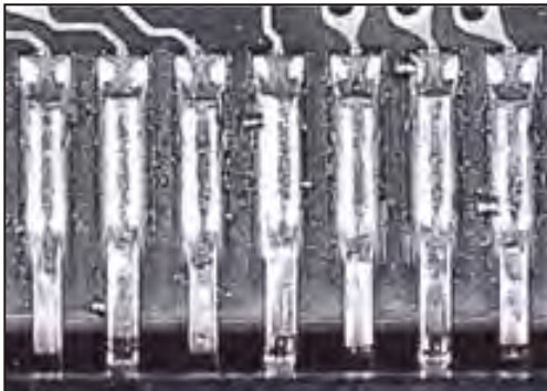
Solder ball spreading test without ZSB
