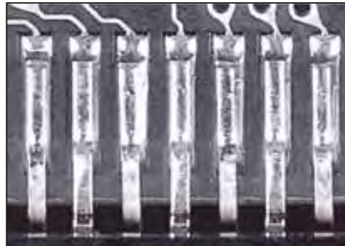
Solder ball spreading test with ZSB
