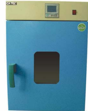
VERTICAL BLAST DRYING OVEN(250°C)
