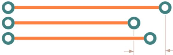
If the third track added is longer than the current longest track, then the rule span now changes and potentially the rule has been violated (because of the increased length):
