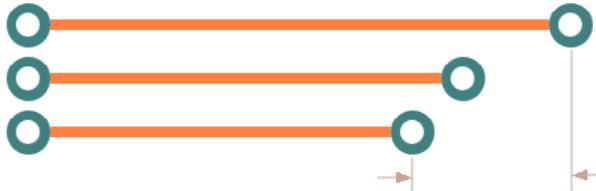
If the third track added was longer than the current shortest track (the middle one) the middle track is still the shortest and the Length Difference hasn't changed:
