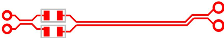
From the **Differential Pairs** dialog you can use the **New Chain** button to define a **Differential Pair Chain**. If your design only contains one pair of defined differential pairs, then selecting this button will display a warning that more than one pair is required.
