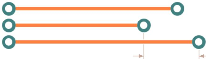
When adding tracks, you should be aware that by default, Pulsonix will treat the longest track as the matched target unless you override this rule using the **Matched Target** check box in the **Rules Spreadsheet** (see below). Therefore, adding a longer track can invalidate existing tracks using this same rule.
