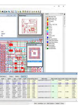
With a clear display of Constraint rules, the High Speed rules spreadsheet dynamically reports values back in real time
