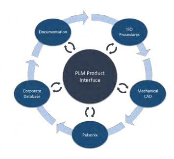
access information within it. Pulsonix has hooks built in which the PLM product can access using the Pulsonix PLM interface. These are programming hooks that are specially written for individual PLM products. For more information about PLM systems supported and the PLM interface, please contact your local Pulsonix service office.
