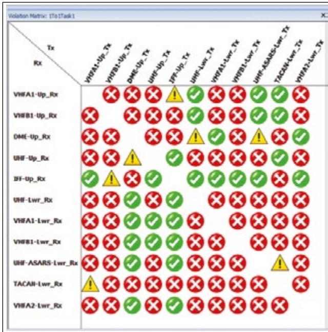
▲ Fig. 2 The Interference Task shows which combinations of RF systems can lead to co-site interference.
